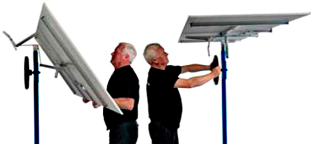
Raise the board and angle the load carrier to the desired angle. Then raise using the knob.
