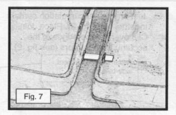
After the tube has moved through both grommets, make sure that the tube is centered approximately between the two accumulation centers (see fig. 9).
