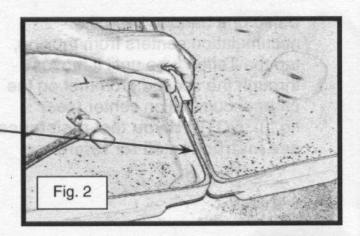
3) Once the Joining Clip is cupped over the top edge of both accumulation centers, proceed to push down the clip with a mallet or small hammer (See fig. 2 and 3). NOTE: Please do not use your hand. Pounding clip with your hand may result in injuries.
