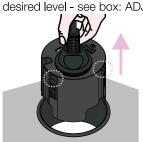
Note! Pay attention to the locking geometry as it will help with adjusting the inner part to the desired level.
