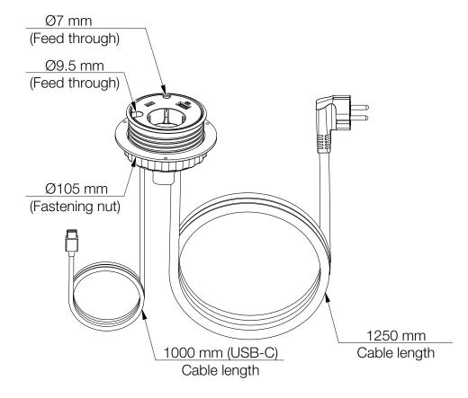
Maximum table thickness: Recommended hole cut: 30 mm Ø79 mm
